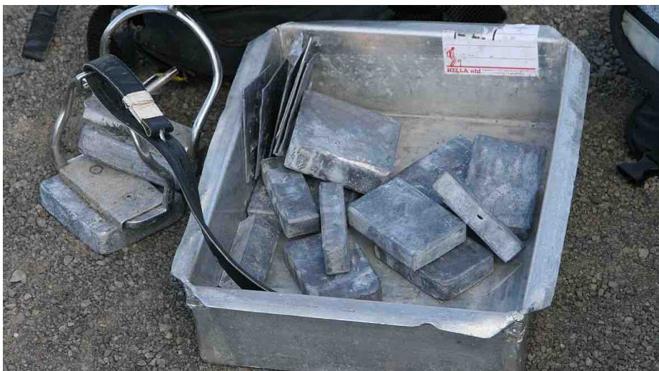
In the tests, Fredrica's weight was systematically changed by adding lead bricks to the saddle (in specially made pouches) or taping them to the stirrups. A lead saddle pad and a lead-weighted vest were used to reach the highest weights, equaling 35% of the horse's body weight. Photo by Sveinn Ragnarsson.
