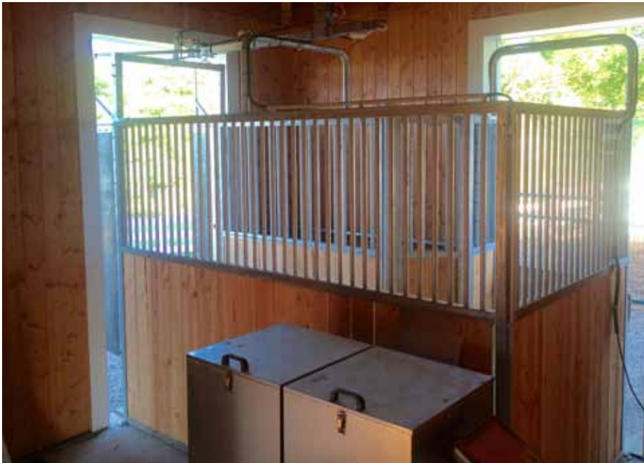
This odd-looking stall is actually an automatic grain feeder designed for the HIT-Active-Stable. A horse with a computer chip tied to its mane (below) can come in up to 10 times a day for a small bit of grain. The owner programs the chip to determine the total daily amount. Photos by Karin Daum.
